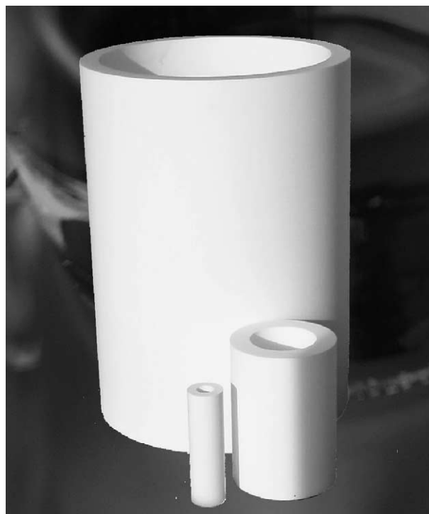
Fig. 1. Shape of CIM tube monolithic columns for radial chromatography in different dimensions (80 and 800 ml are commercially available; the 8000 ml monolith is a prototype).
